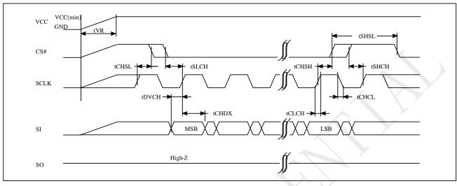
Figure 5-8 AC Timing at Device Power-Up
