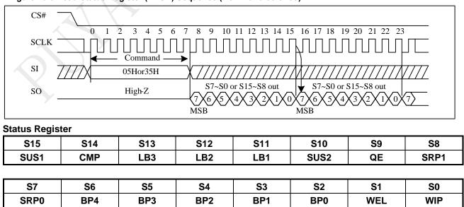
Figure 10-5 Read Status Register (RDSR) Sequence (Command 05 or 35)
