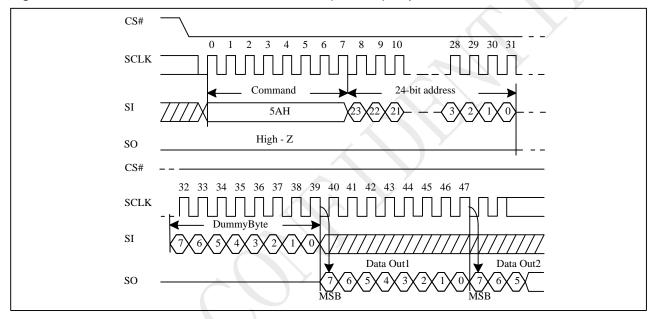
Figure 10-41 Read Serial Flash Discoverable Parameter (RDSFDP) Sequence
